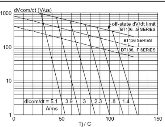
Fig.12. Typical commutation  $dV/dt$  versus junction temperature, parameter commutation  $dI_T/dt$ . The triac should commutate when the  $dV/dt$  is below the value on the appropriate curve for pre-commutation  $dI_T/dt$ .
